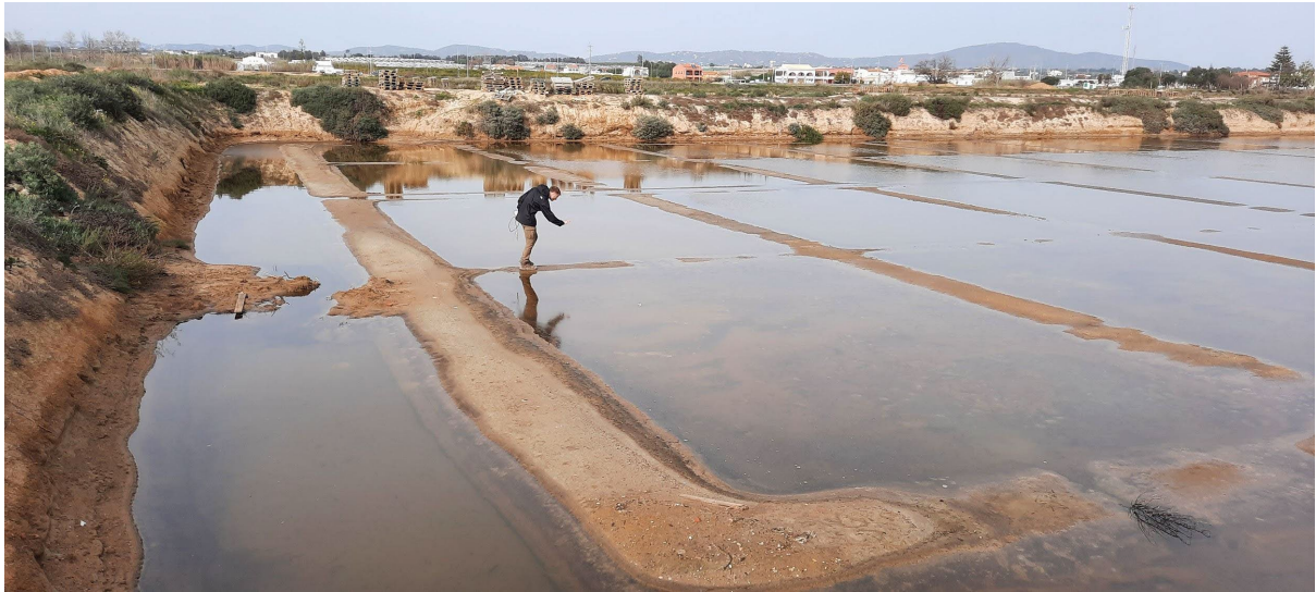
Record high salinity measured in the recently restored Salinas do Grelha, 143 mS, and in one pan the salinity was so high it was not possible to record with the salinity meter (>200 mS)
