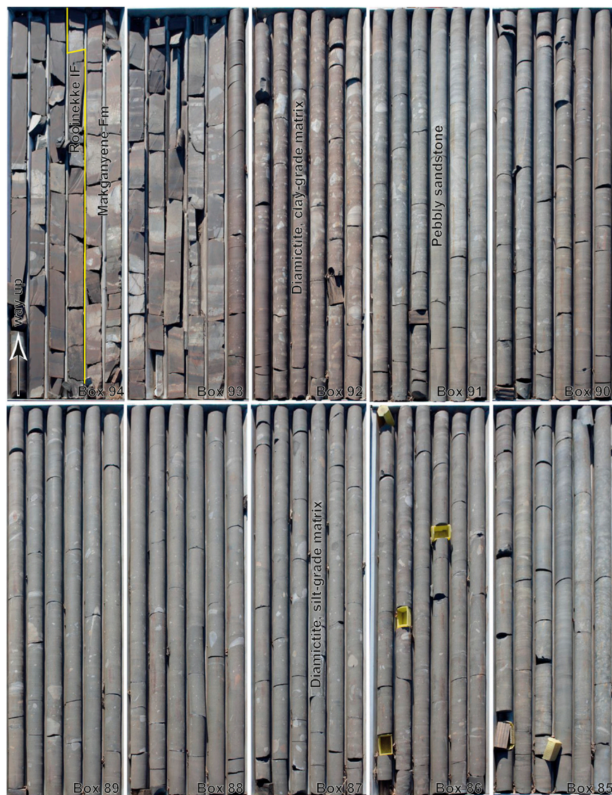
FIGURE 6 Example interval from the HEX 5 core, showing how clearly the facies can be distinguished in contrast to the deeply weathered outcrops.
