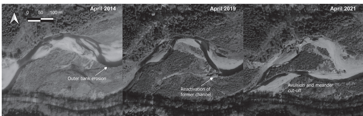
FIGURE 6 Progress of a channel avulsion initiated by flood events in October 2019 and February 2020 at the downstream end of the Grogwynion reach (images: Google 2014 © Maxar Technologies, Google 2019 © CNES/Airbus, Google 2021 © CNES/Airbus).
