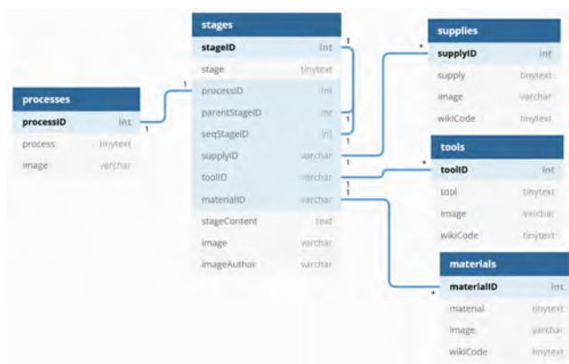
Figure 1: The data model for documenting the processes involved in Islamic woodwork craft.
