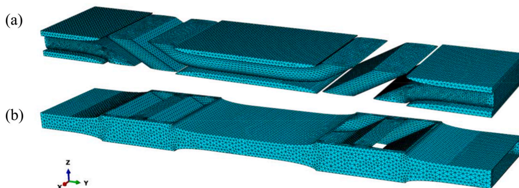
Fig. 7. Typical FE model of a unit cell: (a) tows; (b) matrix constituent.
