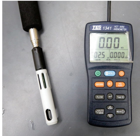
Figure 4. Hot wire anemometer.
