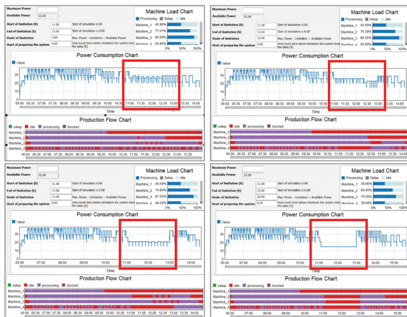
Figure 5. Power consumption and production schedule for scenario 1.
