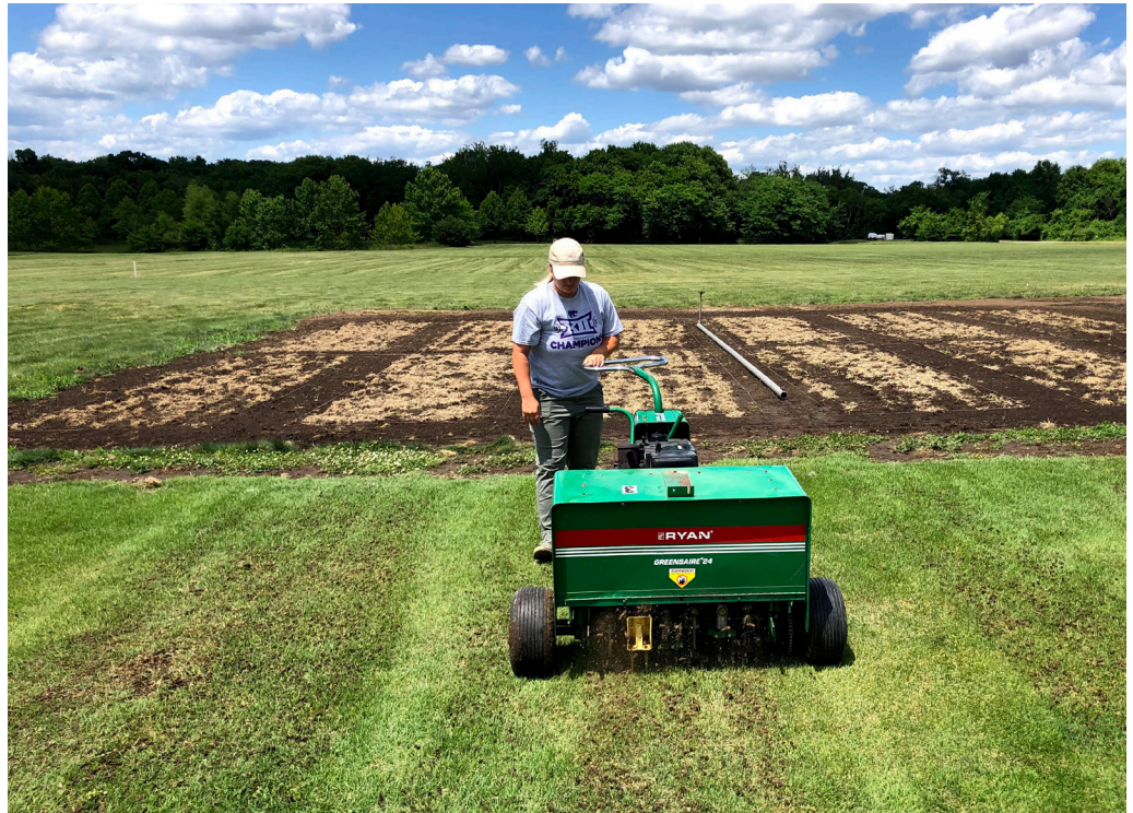
Figure 1. Ryan Greensaire Aerator used to impose aeration treatments on June 21, 2021.
