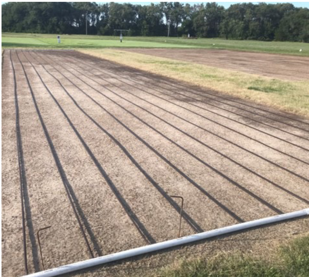
Figure 1. Aboveground drip irrigation system. In this study, driplines were spaced at 18 inches and rested on the soil surface. The subsurface drip irrigation driplines were nearly identical but were buried in the soil at 6 inches.
