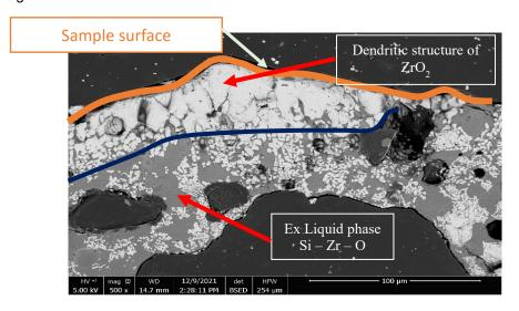
Figure 1 : Oxide structure for a Cf / ZrC – SiC material showing the growing dendritic phenomena after 120s to flame exposition
