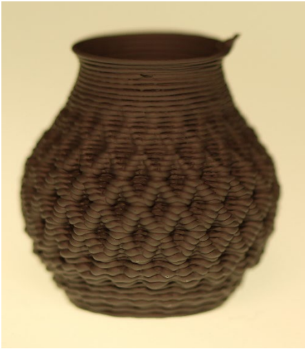
Figure 1: Boron carbide/carbon green body printed through direct ink writing.
