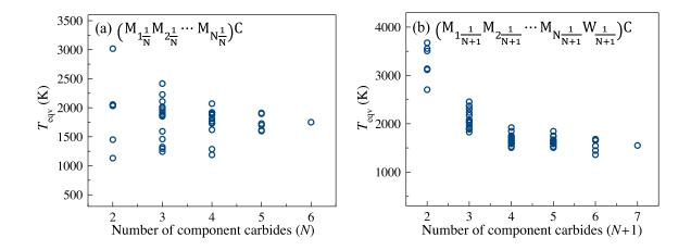
Figure 1: The minimum equilibrium temperature for equiatomic multiple transition element carbide solutions as a function of temperature (a) with and (b) without tungsten.
