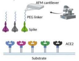
Figure 1: Schematic principle of atomic fore microscopy (AFM) in our setup. The spike protein/glycomuntants is linked to the tip of the cantilever to study interaction forces with the ACE2 glycomutants (both indicated by color codes). These variants are immobilized on the substrate.
