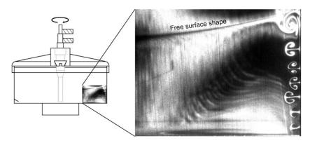
Figure 1 - An example of Taylor-Görtler vortices formed at the wall of a mimic of the CentriCult<sup>™</sup> unit during spin-down to rest, visualised with fluorescent rhodamine dye
