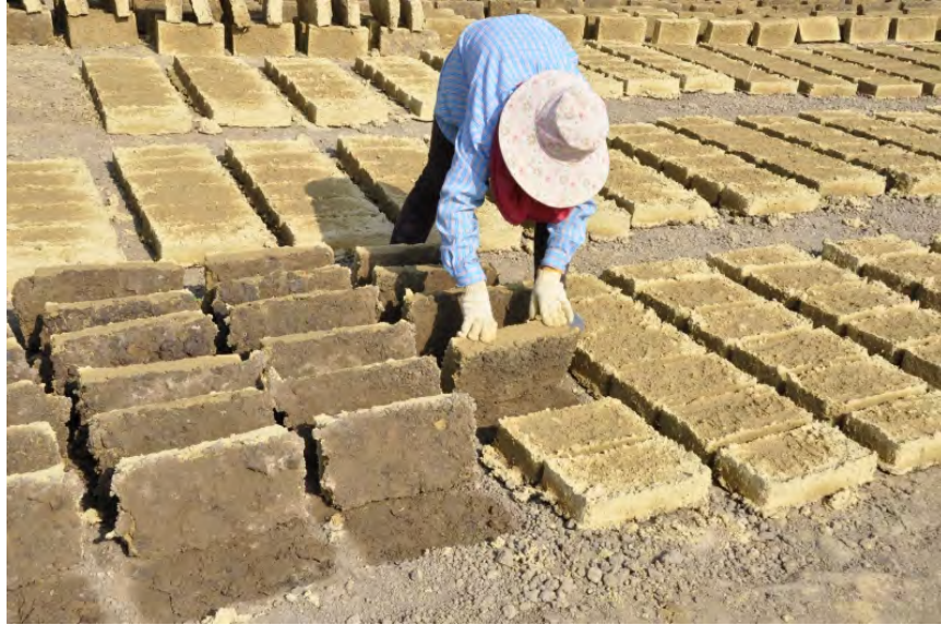
Figure 2.12, CLA CLC, Drying Adobe Bricks at Panyaden School,
