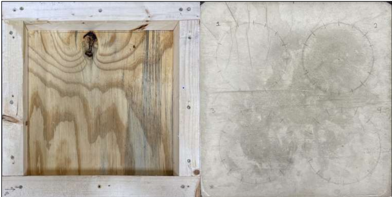
Figure 3.5: A wooden mold (left) and a sample specimen with circle markings (right)
