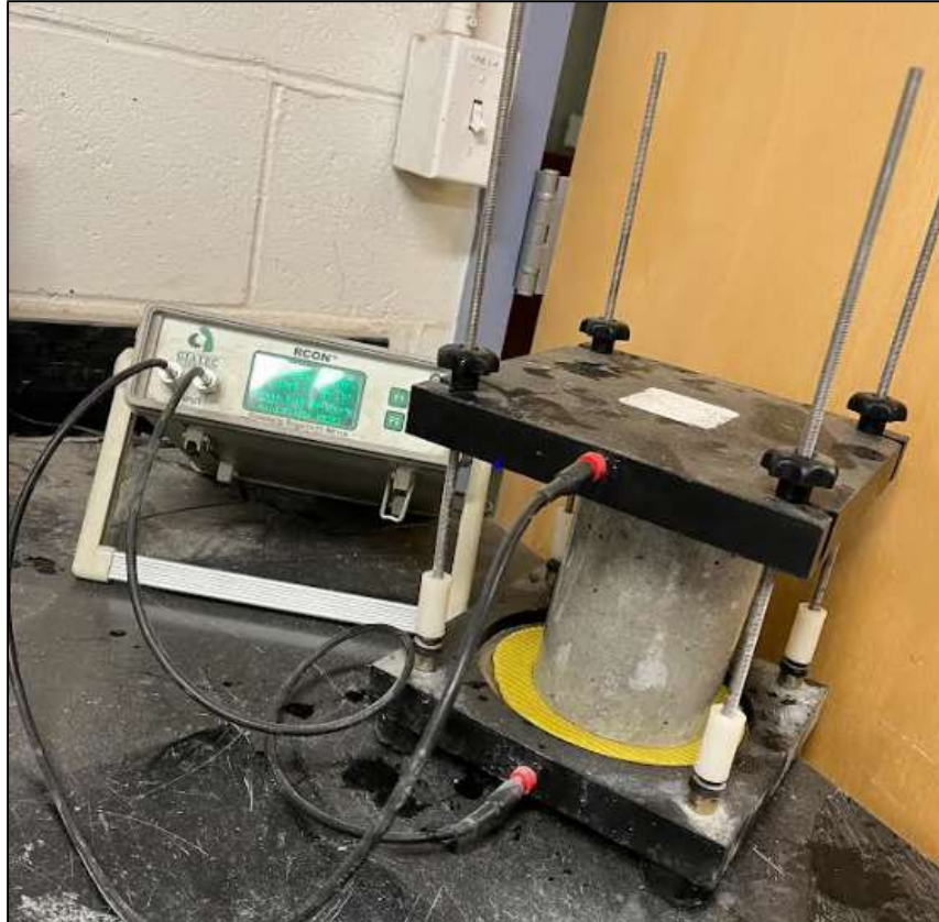
Figure 3.11: Setup for RCON2 bulk resistivity meter
