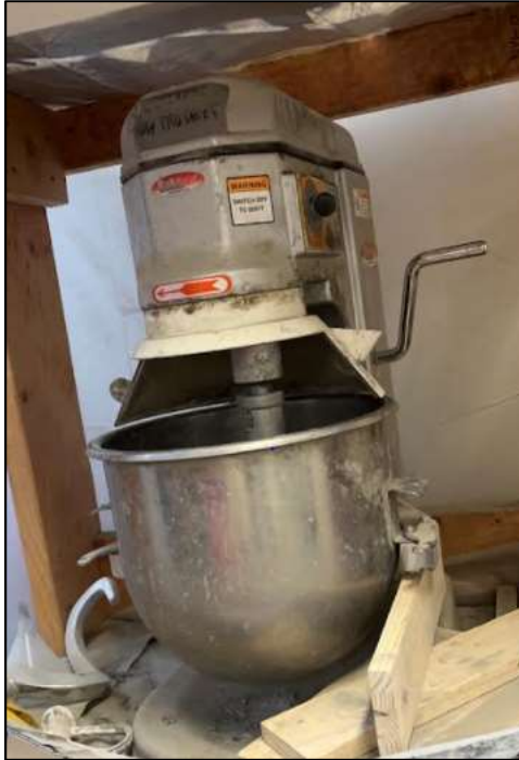
Figure 3.4: The BakeMax planetary mixer setup for mixing HPC
