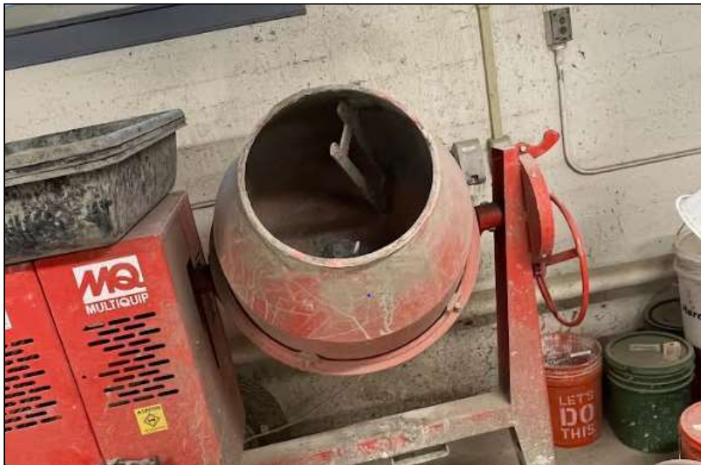
Figure 3.10: Mixer used for creating concrete specimens
