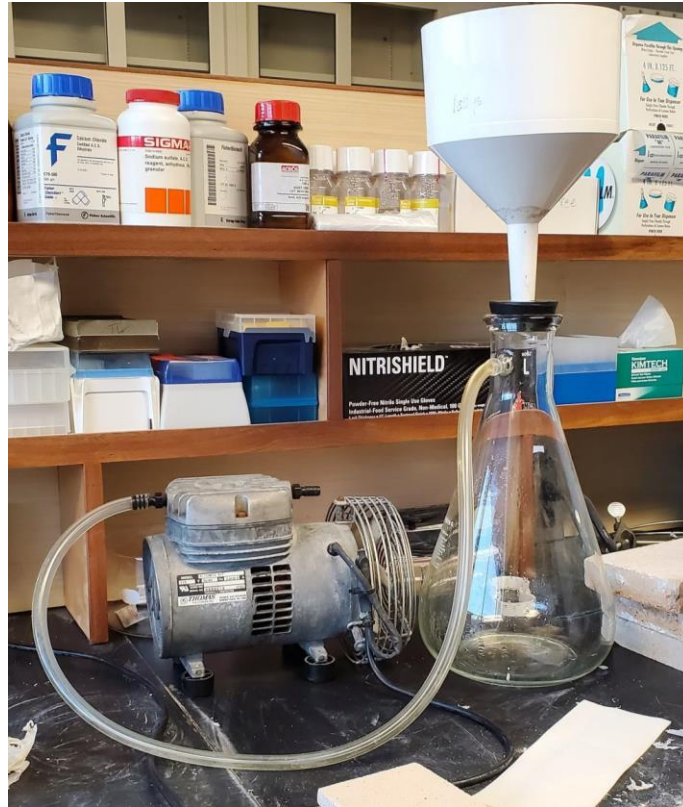
Figure 5.1: Vacuum Filtration Setup for Dilute Mixed CNF.
