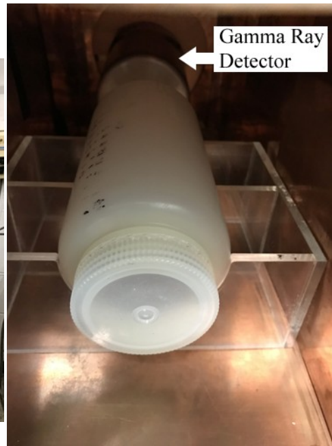
Figure 2.4, Left: The horizontal gamma ray detector used in counting all air filters, showing the shield from the outside. Figure 2.5, Right: The interior of the shield, showing the detector and nalgene bottle.
