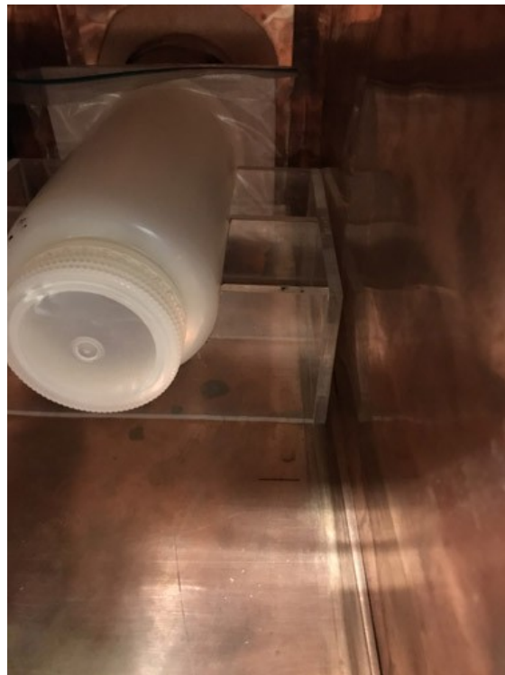
Figure 2.6, Left: Air filter in its wax paper envelope, mounted on the nalgene bottle for counting.
