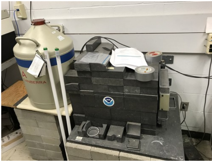
Figure 2.4, Left: The horizontal gamma ray detector used in counting all air filters, showing the shield from the outside. Figure 2.5, Right: The interior of the shield, showing the detector and nalgene bottle.
