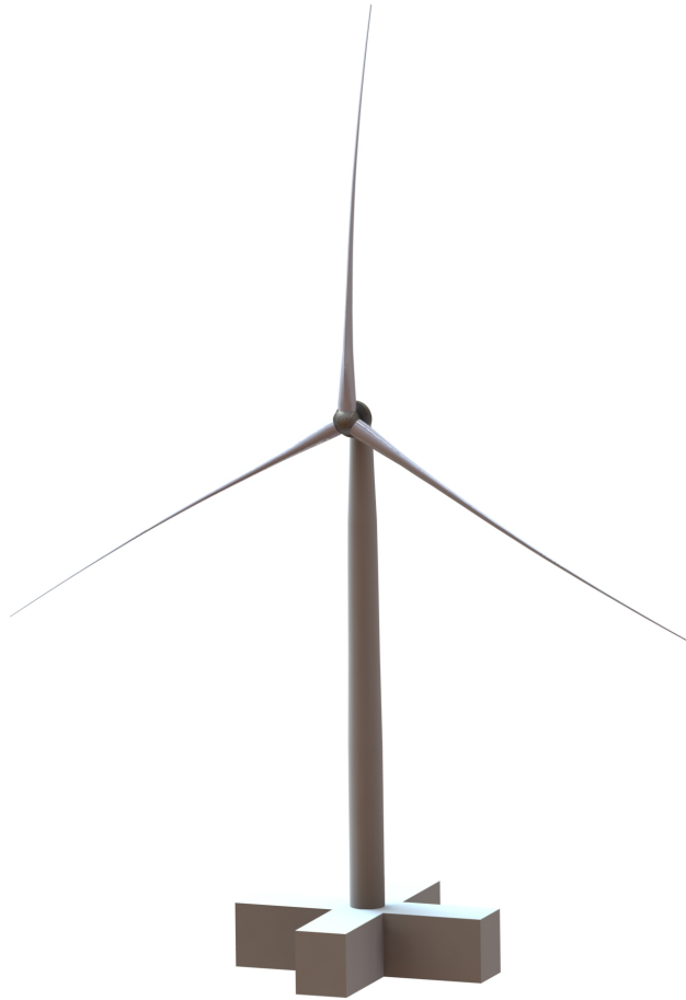
Figure 3.1: Rendering of the converged platform with the IEA 15 MW turbine
