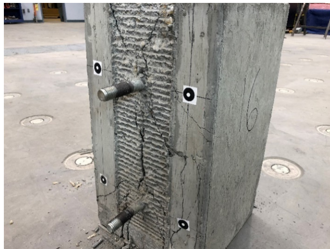
Figure 8. Compression-Shear Specimen after Loading to Failure.
