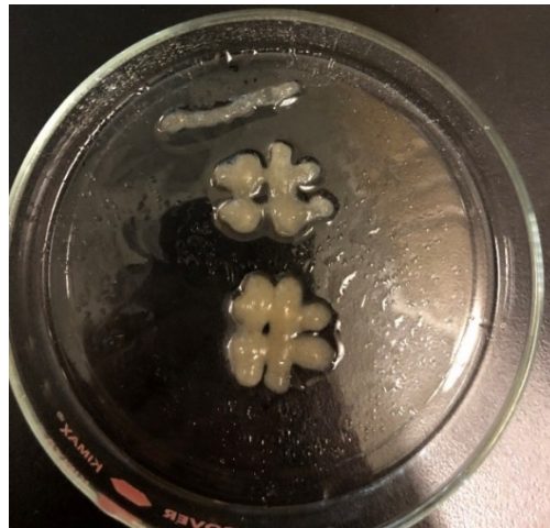
Figure 8. Syringed structures of 3:1:1 w/v% ink; line is at the top, the single layer hashtag is in the center, and the triple layer hashtag is at the bottom.
