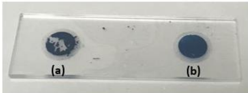
Figure 2.7. The photograph image of the (a) Non-uniform distribution of PAMB particles obtained after passing 12 mL of PAMB suspension of 100 \mu\text{gL}^{-1} phosphate solution through a 0.45 \mu\text{m} pore membrane. (b) Uniform distribution of PAMB particles was obtained over the membrane after passing 6 mL PAMB suspension of the same 100 ppb phosphate solution through a 0.45 \mu\text{m} pore membrane.
