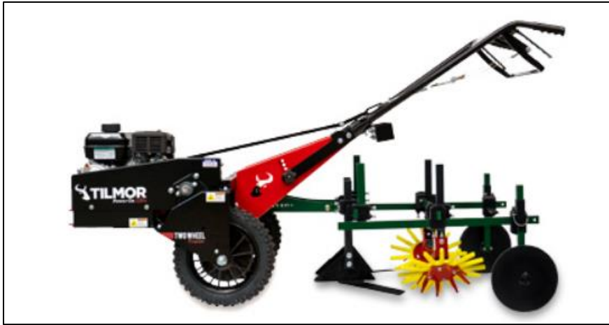
Figure 1. 1. The Tilmor Power Ox, a walk-behind tractor option for small-scale farmers. It can be equipped with implements such as sweeps and finger weeders (pictured above), which can be adjusted to kill weeds in the crop row. Source: Tilmor.
