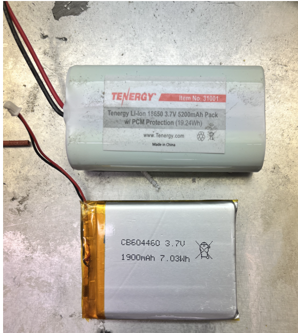
Figure 3. A comparison between the smaller 1900 mAH battery and the larger 5200 mAH battery.
