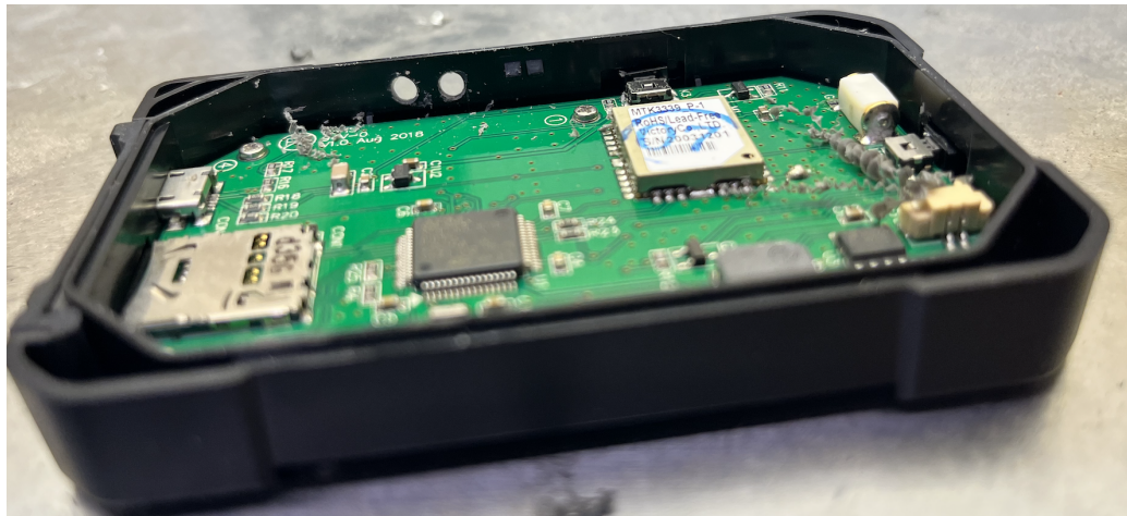
Figure 4. The motherboard of the GPS, showing the two drill holes in the sidewall where the wires for the 5200 mAH battery were put through to connect it to the GPS.
