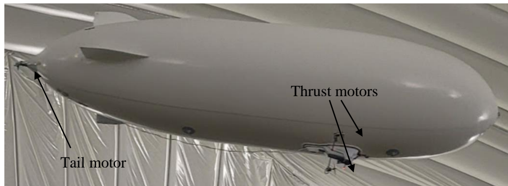
Fig. 10. A picture of the propulsion elements.
