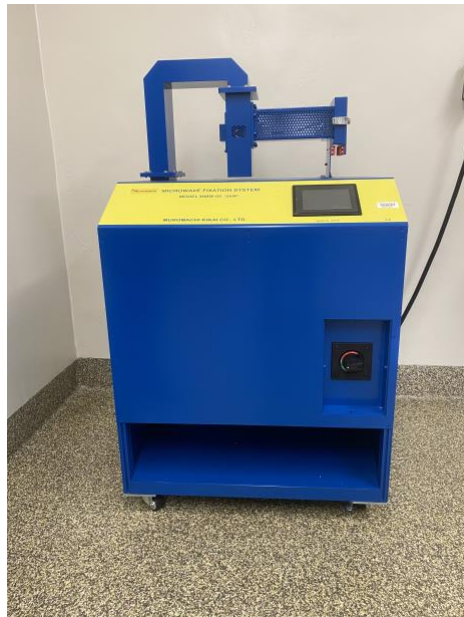
Figure 2.6 Muromachi Kikai Company High Power Focused Microwave.
