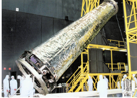
Figure 1.4: Assembly of the Chandra telescope.
