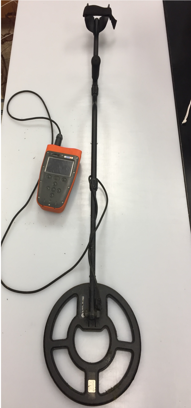
Figure 7: Biomark HPR Plus portable PIT tag reader and Biomark BP Portable Antenna Plus used to conduct PIT telemetry surveys.
