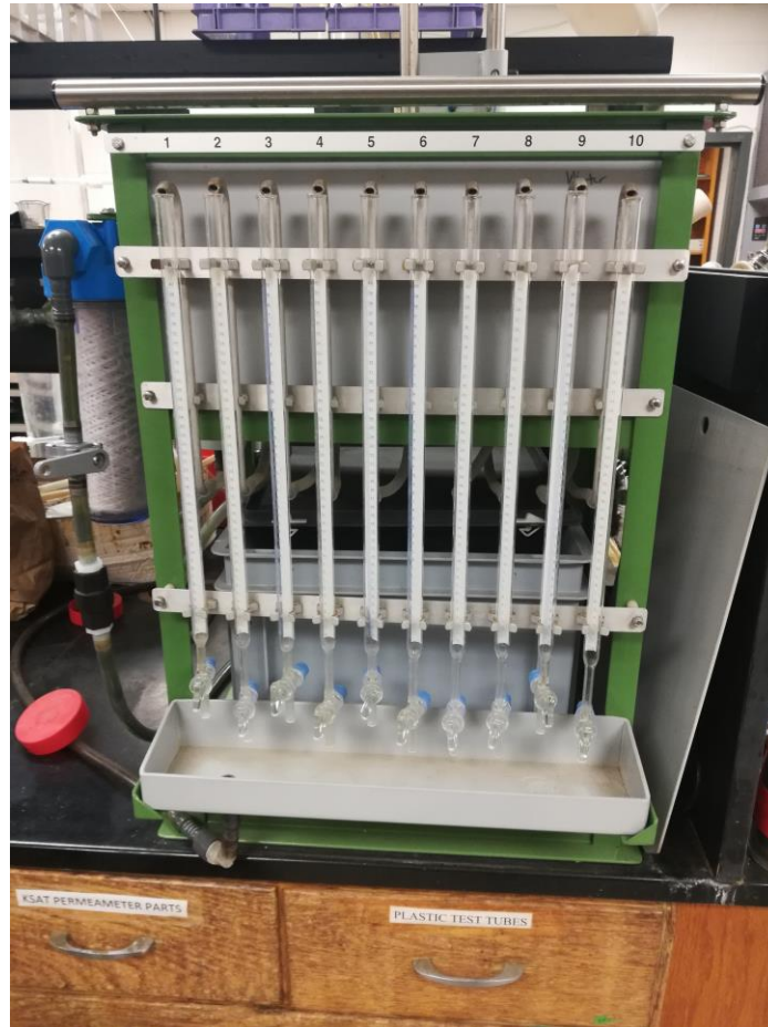
Figure B. 1. The Eijkelkamp laboratory permeameter used to measure saturated hydraulic conductivity.
