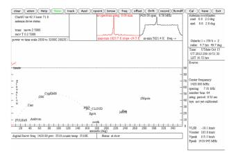
**Fig 2:** Interface through which the telescope is controlled. The graph on the left shows the instantaneous RF, and the graph on the right is integrated over time. Image taken by Eric Gustafson in 2012.
