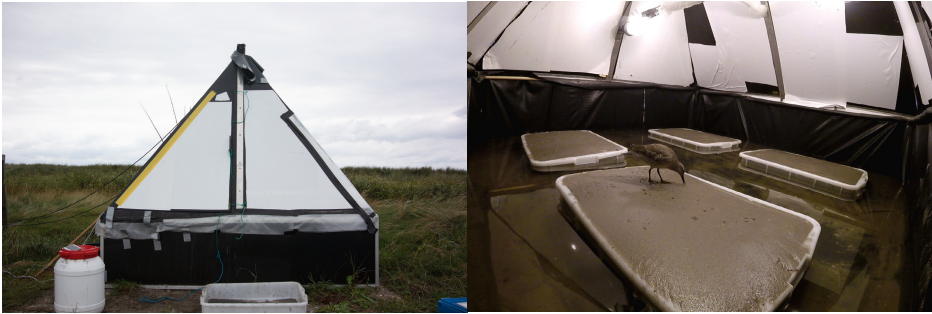
Figure 4. Mobile tent setup to score exploratory behaviour at the field site. The floor of the unit consists of sea water of 20 cm height and 4 identical sand patches 61cm x 40cm for birds to explore, tent measures 2m x 2m x 1m.
