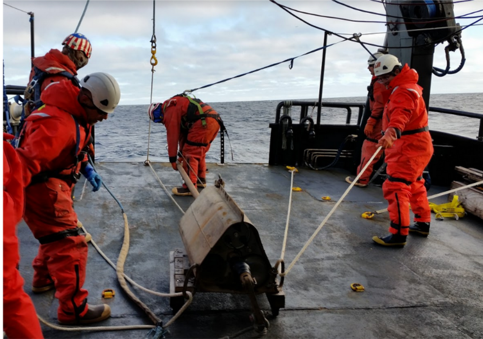
Figure 2: Lister probe on the deck of a ship before deployment via A-Frame. Image courtesy of Matthew J. Hornbach, taken during heat flow study in the Beaufort Sea.
