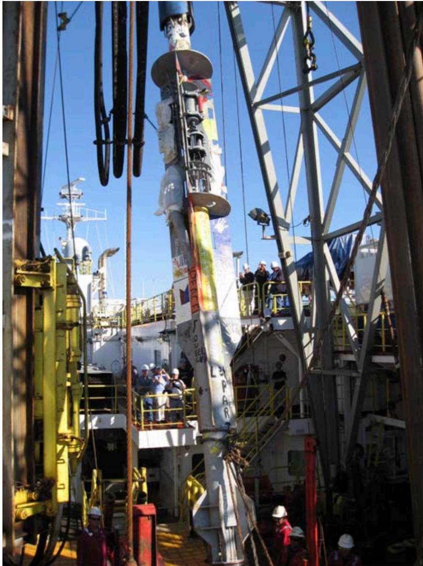
Figure 3: A CORK system. Picture originally published in “Design, deployment and status of borehole observatory systems used for single-hole and cross-hole experiments IODP Expedition 327, eastern flank of Juan de Fuca Ridge” [14]
