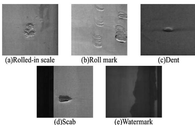
**Figure 2** Surface defects image of steel plate
