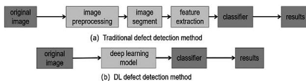
**Figure 3** Comparison of the traditional defect detection method and the DL defect detection method
