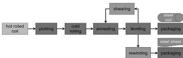
**Figure 1** The process of cold rolled steel plate
