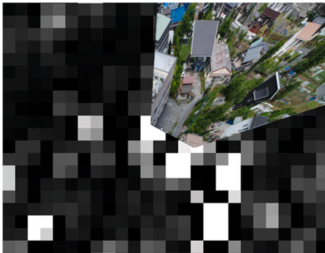
Fig. 24. Registration result between SAR and ground-level shooting images. It can be seen that areas where retroreflections occur, such as buildings, are represented by bright pixels.
