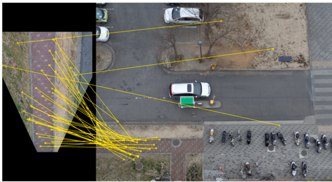
Fig. 13. Detecting corresponding points between virtual top-view and low-altitude images.
