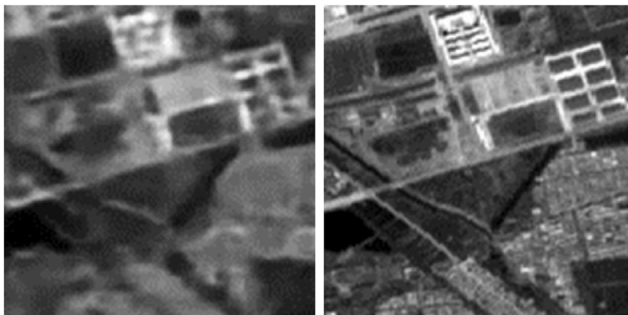
Fig. 3. Generated image by conventional cGAN (left) and the answer image (right). Left image, the blur smooths out the luminance gradient, which loses accuracy of the corresponding point detection.
