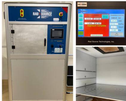
**Figure 9: X-Ray Irradiator.** RS 2000 X-ray Biological Irradiator was used to irradiate macrophages. The following parameters were set: 160 kV, 25.0 mA, Configuration: Shelf Only, Shelf Level: 3, Radiation: 7 Gy, Exposure Time: 3 mins 36 secs.
