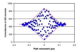
FIG. 2. (Color online) Data points depict the typical interference envelope which is observed in the coincidence rates of the Franson interferometer as a function of path mismatch. The solid line is the theoretical triangular envelope function which is calculated for a square biphoton wave function of coherence time  $\pi/\Omega_f$ =100 fs.
