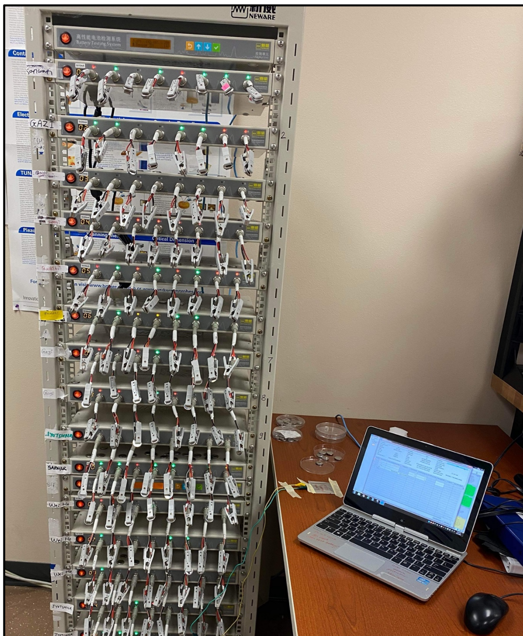
Figure 8: Neware battery analyzer
