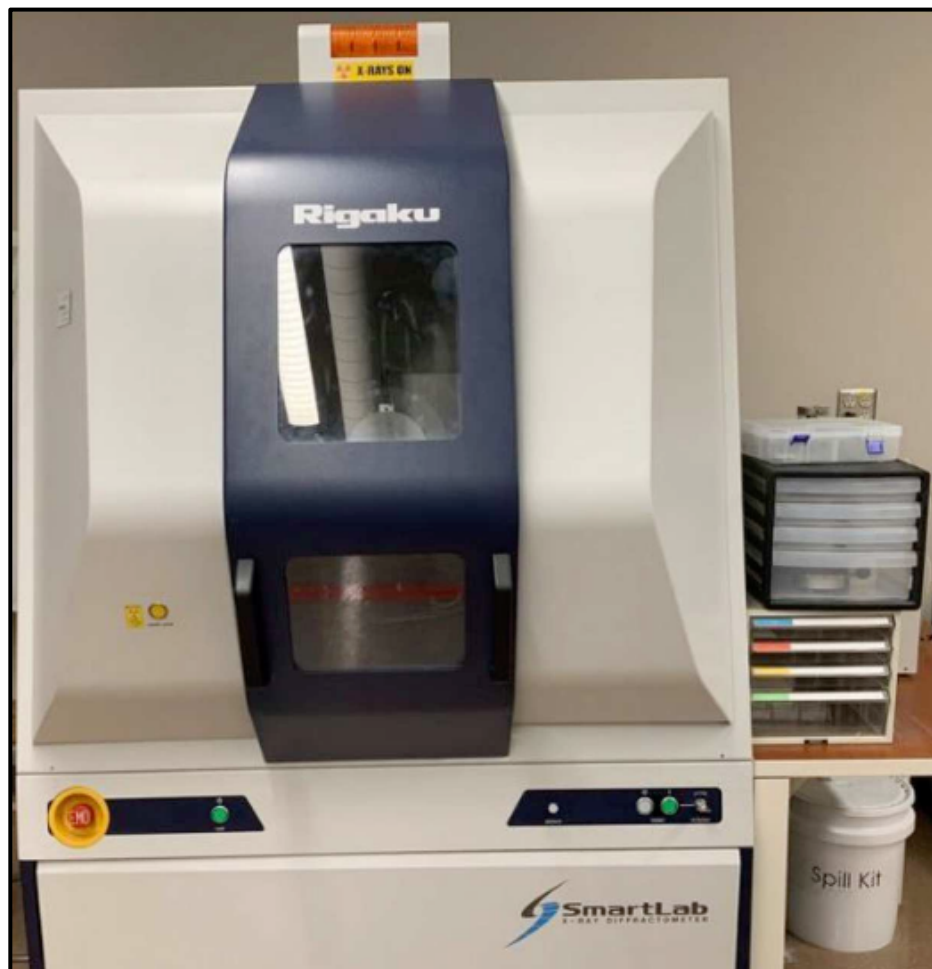
Figure 5: Picture showing the X-ray diffractometer located in the Lab at SDSU.
