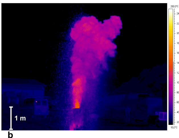
Fig. 2 Thermal images of a high temperature run forming a buoyant plume. Temperatures are in ^{\circ}\text{C} . a Formation of the eruptive column at conduit exit. b Spread of the column and thermal convection
