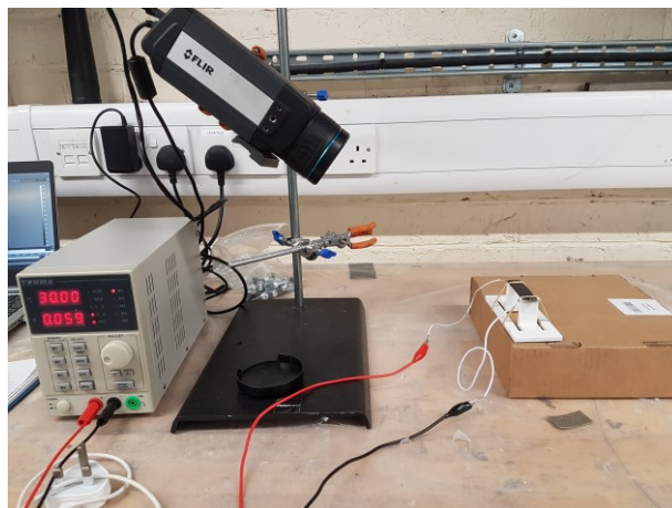
Figure 1: Experimental set-up for Joule self-heating investigation
