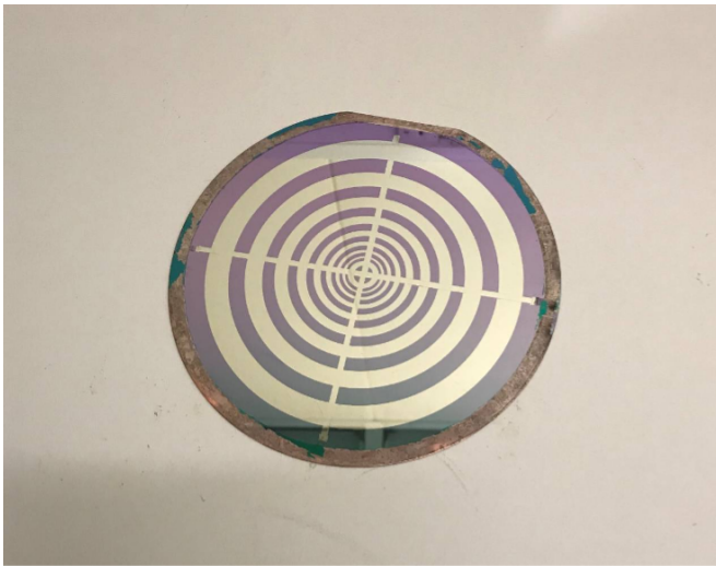
Fig. 6. 150 mm wafer with dummy current structures (5nm Al / 5nm Ni seed).
