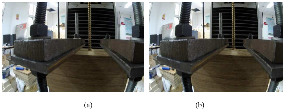
264 Fig. 7. Specimens under loading: (a) Initial stage of loading, (b) Approaching peak load
