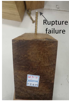
Fig. 6. Rupture failure of the STSs for \lambda=7.5
