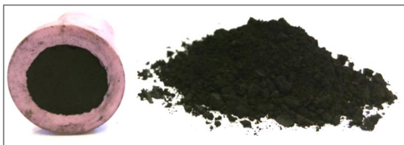
Fig. 6. Samples of CuO prepared to be introduced into the solar reactor: packed sample to be used under static working mode and powder sample to be used directly under rotary working mode.
