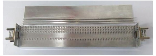
Fig. 9. Gap waveguide leaky wave antenna prototype.
