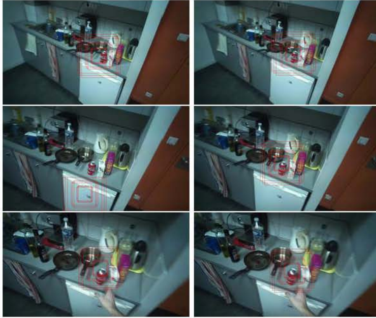
Figure 5: An illustration of Noise Reduction technique. (Left) Frames with candidate ROIs computed over the original sequence of gaze points. (Right) Noise-free candidate ROIs by back-projecting the predicted object location to the frame sequence.
