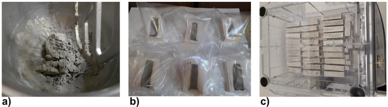
Figure 2. Mixing (a) and curing (b-c) of cement-based mortar samples.
