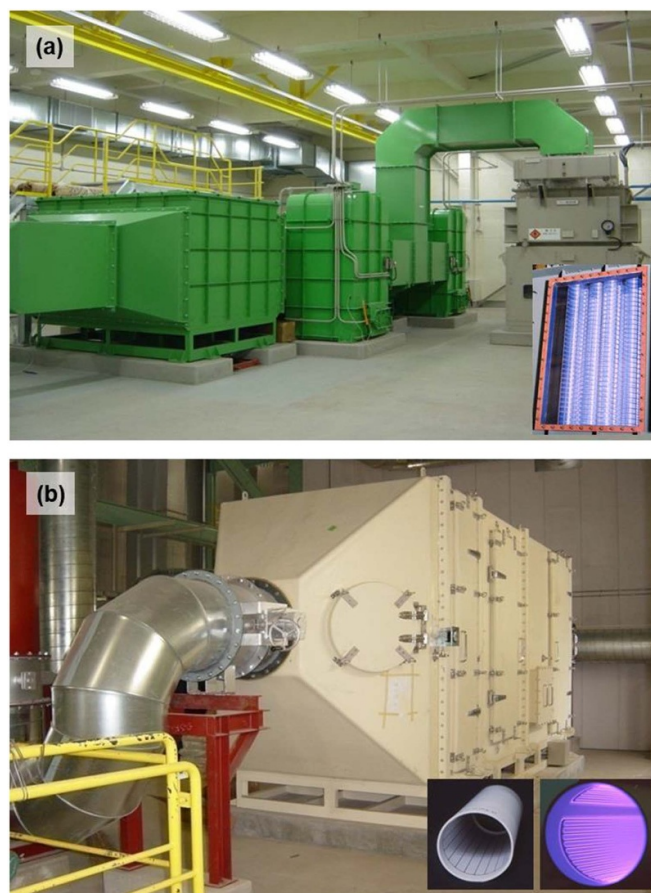
Figure 21. Large-scale application of plasma deodorization facilities in Japan: (a) pulsed plasma chemical process with 30 000 nm 3 h -1 processing capacity (b) surface plasma chemical process with 9500 nm 3 h -1 capacity. Reproduced with permission from Dr Hosokawa of Masuda Research Co.
