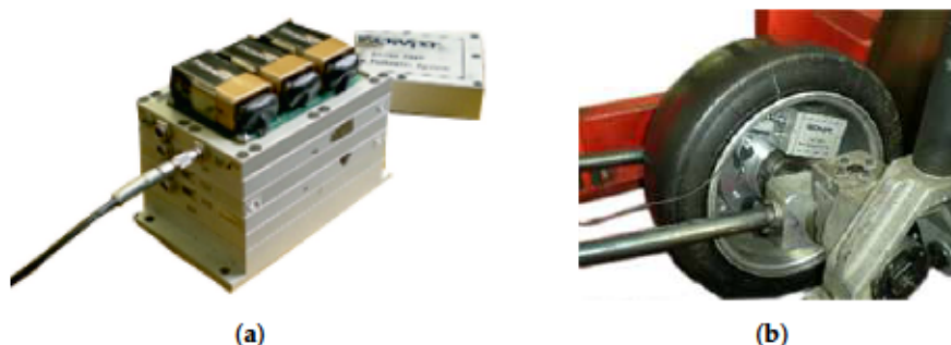
Figure 3. Acquisition system SoMat ® 2000: (a) Microprocessor for the data acquisition, and a Power/Communication module; (b) Data acquisition module installed on the tire [28].
