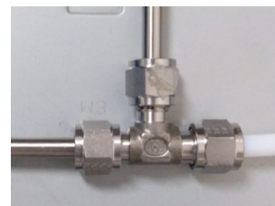
Fig. 2. Photograph of the piping joint employed in the proof-of-concept experiment.
