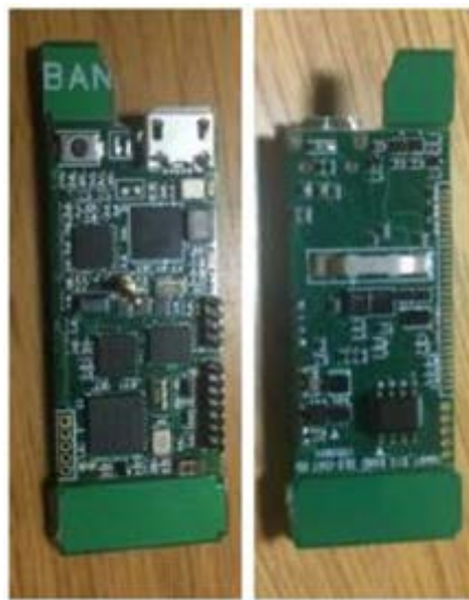
Figure 4.4: Main module for the prototype, without electrodes and battery.
