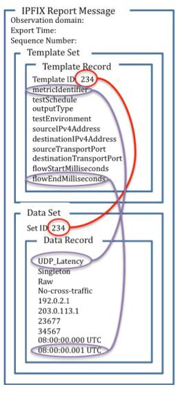
Figure 4: Example of an IPFIX report message for a UDP Latency test
