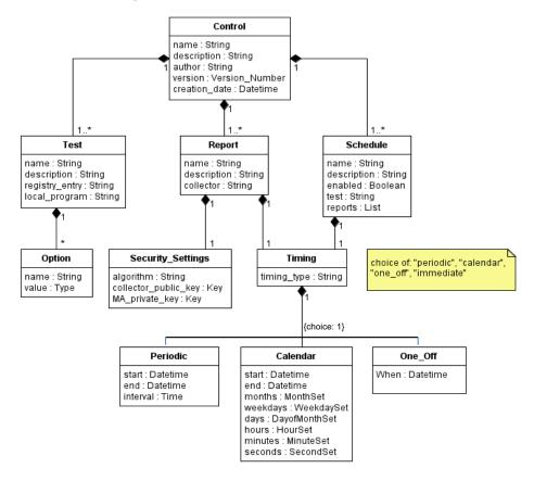
Figure 2: Proposed Information model for the control protocol, in UML
