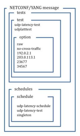
Figure 3: Example of a NETCONF/YANG control message for a UDP Latency test
