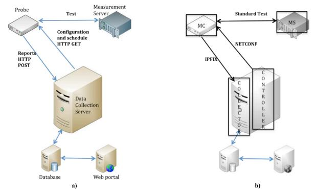
Figure 1: Measurement platform architecture. Figure 1.a) shows the current SamKnows architecture, whilst in Figure 1.b) the proposed reference architecture is overlaid on top of the SamKnows architecture.
